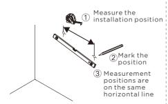
•1. Select the installation location of the floor cabinet on the wall, then use a pen to mark the drilling location, and use a level to ensure that the holes are on the same horizontal line. (The recommended installation height of the floor cabinet is 800-850mm. Please customize the installation location according to the actual situation. The smart model needs to reserve a power supply
