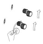
2. Wrap the elbow with PTFE tape, then connect it to the pre-embedded water outlet pipe joint.
