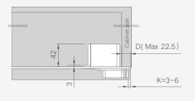
D=Required door overlay K=Drilling distance of hinge cup
