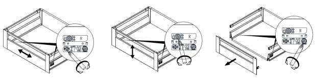
Front panel side adjustment ± 1.5mm
