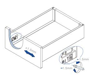
9 Front panel disassemble
