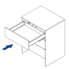
① Drawer and slide disassemble
