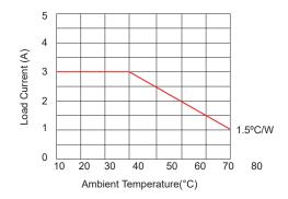
Note: This product can be installed on a panel with a thermal resistance of  $\leq 1.5$  °C/W to assist in heat dissipation.
