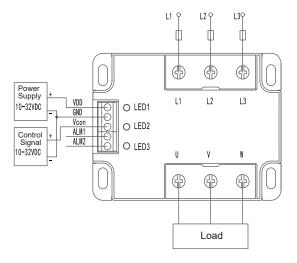
VDD: External DC power anode (10-32VDC)
