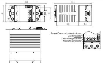
Power supply/Communication indicator: LED lights up when there is a power supply;
