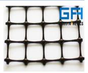
This traffic loading is transferred to the geogrid by the interlocking action of the granular aggregate within the apertures of the biaxial geogrid and the frictional resistance generated between the geogrid and sub base. GeofanGrid PPDN offers very low elongation of 13-15% at ultimate load capacity, but more importantly the high modulus of the material means low elongation when initially loaded, thus reducing rutting, road wear and ultimately increases the design life of the road structure.
