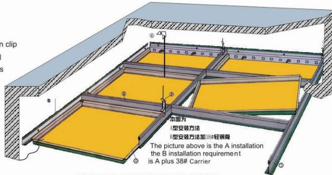
本图为 A型安装方法 B型安装方法加38#轻钢骨 The picture above is the A installation the B installation requirement is A plus 38# Carrier
