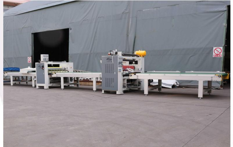
This machine is specialized for lamianting the transparent arylc sheet with the thin PVC, it can make many diffence patten,colour acrylic sheet.
