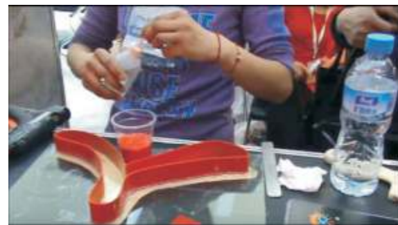
Add the hardener (B) into the Epoxy resin (A) with colors
