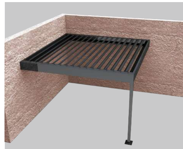
Install On A Right-angled Wall (2 Walls) 1 post
