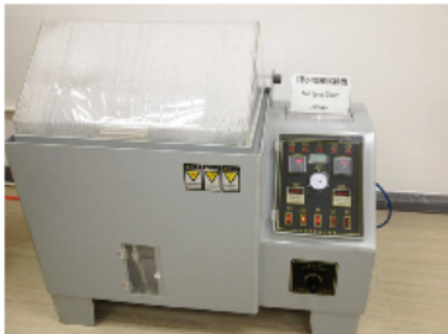
Swing test equipment Salt spray test equipment
