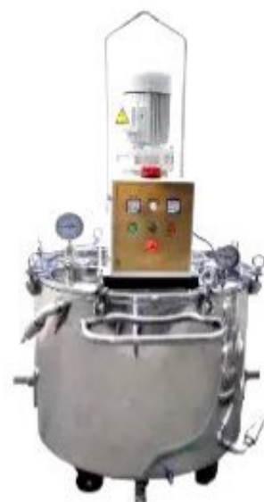
Slurry Transfer Tank
