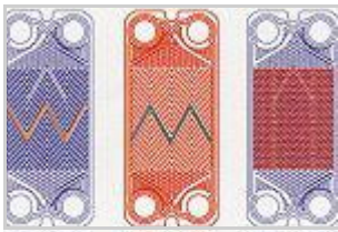
Low angle channel arrangement For lower allowable pressure drop requirement applications
