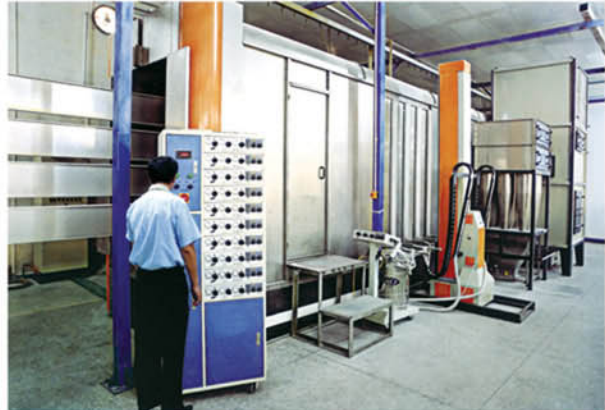
瑞士金马全自动喷涂生产线控制台 Console for the automatic spraying production line of Swiss Gema brand
