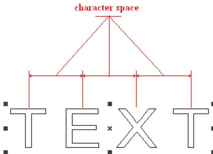
Figure 4-31 Calculate spacing according to character center
