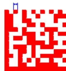
Figure 4-23 Data Matrix Barcode Width
