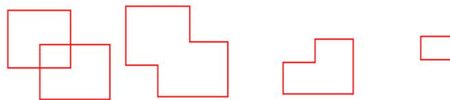
Figure 5-10 Plastic 1. Original 2. Joint 3. Shear 4. Intersect
