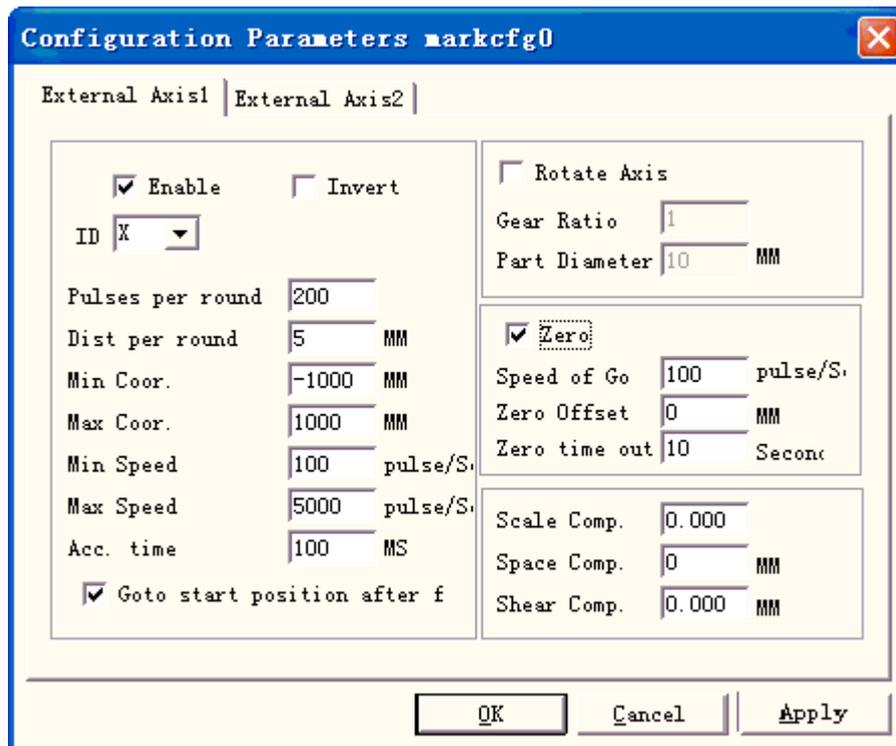
Figure 8-33 configuration parameters of expansion axis
