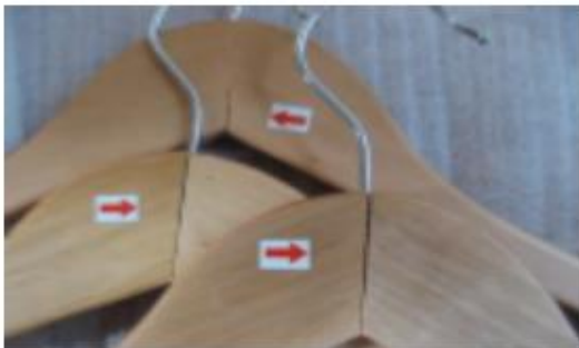
X joint crack is refuse
