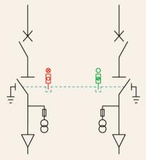
V circuit breaker cabinet T w o in c o m in g lines+contact cabinet interlock (Three locks and two keys)
