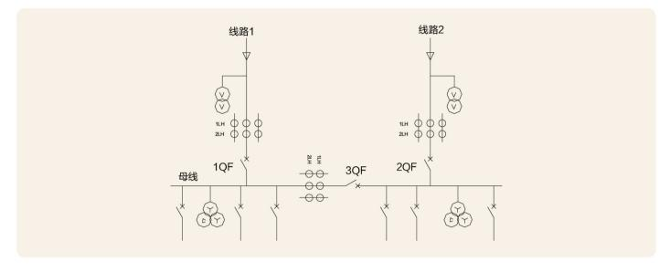
Power switching between 2 incoming lines (1QF and 2QF) and bus tie switch (3QF). 4 working modes (can be selected from the MIC500 unit)
