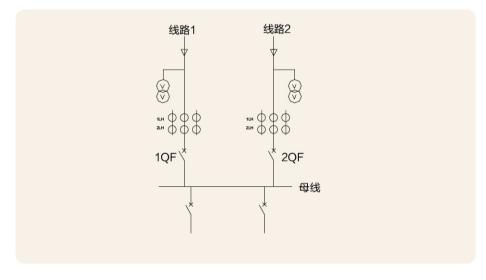
${\sf I}_{\sf V}$  IQF automatic charge and automatic recovery or 2QF automatic charge and automatic recovery mode
