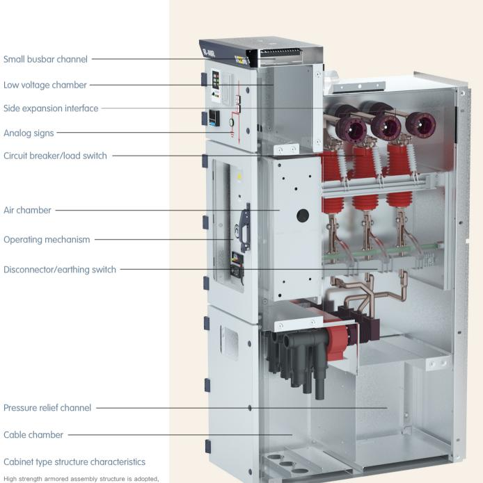
High strength armored assembly structure is adopted, and the aluminum zinc coated steel plate is precision processed by CNC process
