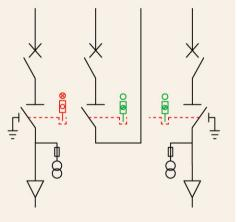
Locking transformer door of circuit breaker cabinet (two locks and one key)
