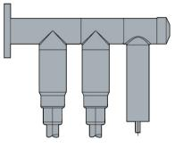
Assembly drawing of front plug, rear plug and arrester
