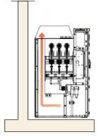
Metering cabinets mounted away from the wall, or against the wall
