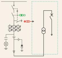
Circuit breaker cabinet locks the low-voltage side circuit breaker of transformer (two locks and one key)
