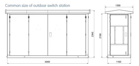
Outdoor box width: The sum of the width of a single ring network cabinet + DTU width (standard 600mm) + reserved space (400mm) Outdoor box height: <2450mm Outdoor box depth: 1150mm
