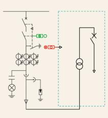
Circuit breaker cabinet locks the low-voltage side circuit breaker of transformer (two locks and one key)
