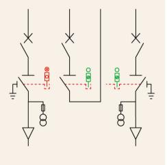
Locking transformer door of circuit breaker cabinet (two locks and one key)
