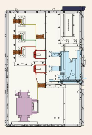
NXSAFE-F Combined switchgear of load switch fuse
