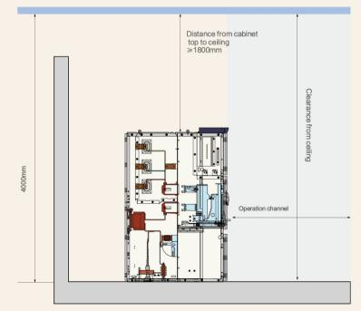
Minimum operating clearance channel in front of the switch cabinet when the switch cabinet is against the wall (m)
