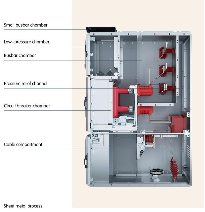
High-strength corrosion-resistant aluminum and zin plated plates go through CNC machining equipment's sheet metal process and are assembled with high precision double-flanged process, and connected with high-strength bolt and rivet to guarantee the cabinet's precision and strength.
