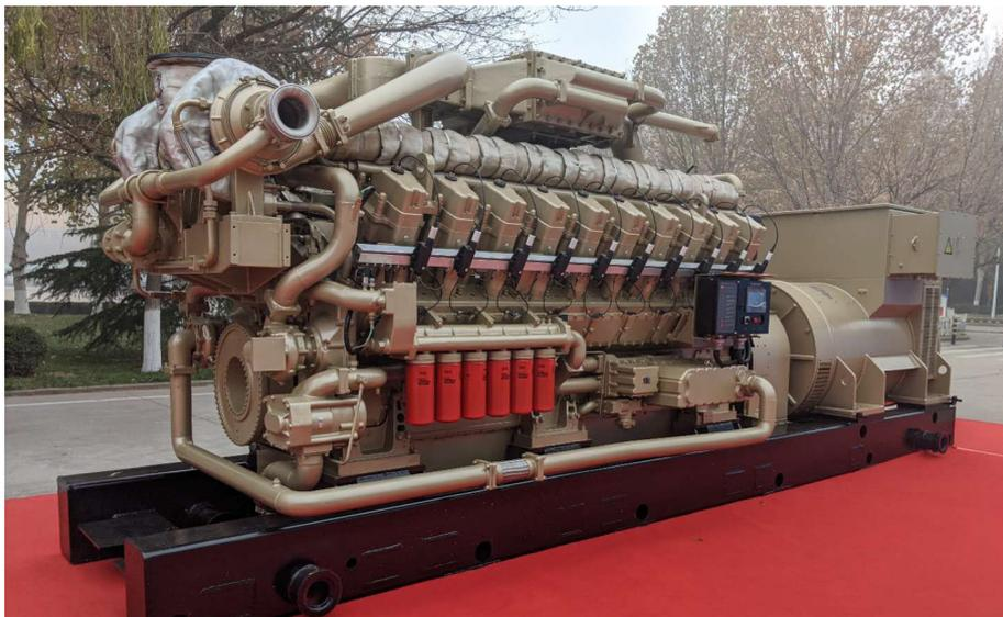
L20V190 gas engine genset adopts world advanced close cycle air-fuel control system, lean burn, millar cycle, high energy intelligent ignition and pre-burn chamber spark plug etc. technology, which makes the engine high power performance and economical. The average efficiency pressure reaches 1.83mpa, heat rate is lower than 9000 k/kwh.
