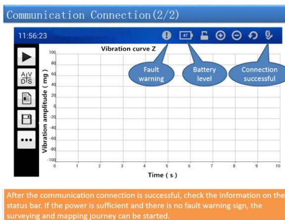
**Figure 2.7 successful connection, status display**
