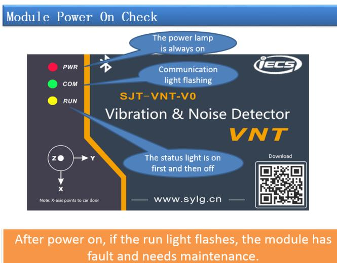
Figure 2.5 power on inspection
