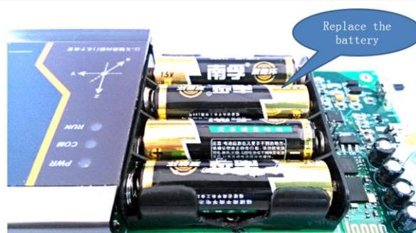
After replacing the battery, install the module according to the above reverse order, and pay attention not to damage the internal components.
