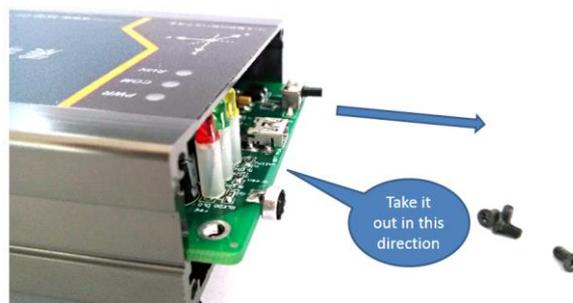
Take out the circuit board along the slide and be careful not to damage the device.
