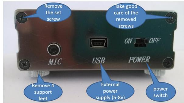
After unscrewing the four fixing screws of the side panel and the four supporting feet at the bottom, open the side panel
