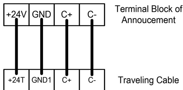
Figure 4 Wiring Diagram
