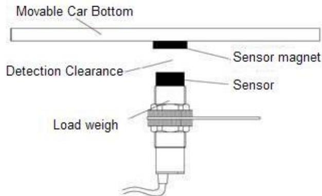
In the site, if the range of car bottom movement beyond 10mm, you can change No load test point to over 10mm (Less than 20mm).
