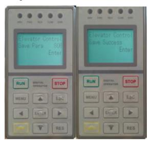
After saving parameter, disconnect WCR from motherboard, waiting for complete discharge (about a few minutes, the power light is off.) and then reconnect.
