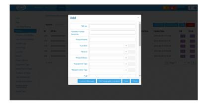
Step 6 Add alarming man. On the "SMS Setup" page of the monitoring platform, fill in the mobile number of the person who will be attending the breakdown. When elevator has breakdown, the system will send the error message via SMS to the alarming man. It is possible to send a test message to the alarming man, if he receives the message that means the sending message is normal.
