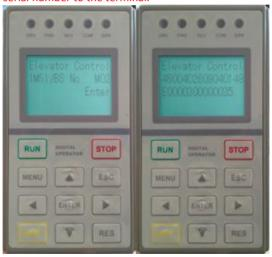
Step 5 Add elevators to platform. Enter 'System' – 'Elevator' page on GEMS system, click "ADD" and fill in BS No. which obtained in step 4,the columns with "\*" must be filled in.
