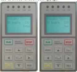
Set IP address of WCR remote monitoring platform: Find remote monitoring platform IP address setting page by flipping through all pages, press 'ENTER' to enter the page, set IP address as 'wcr.fuji.com.sa', then press 'ENTER' again to complete the setting, finally press 'Esc' to exit IP address setting interface.
