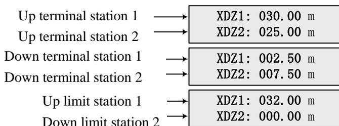
(3) Press  $\wedge$  and  $\vee$  keys to change the observation item in hoistway switch position interface. Press Esc to return.
