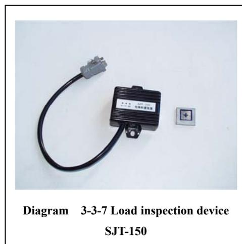
Diagram 3-3-7 Load inspection device SJT-150
