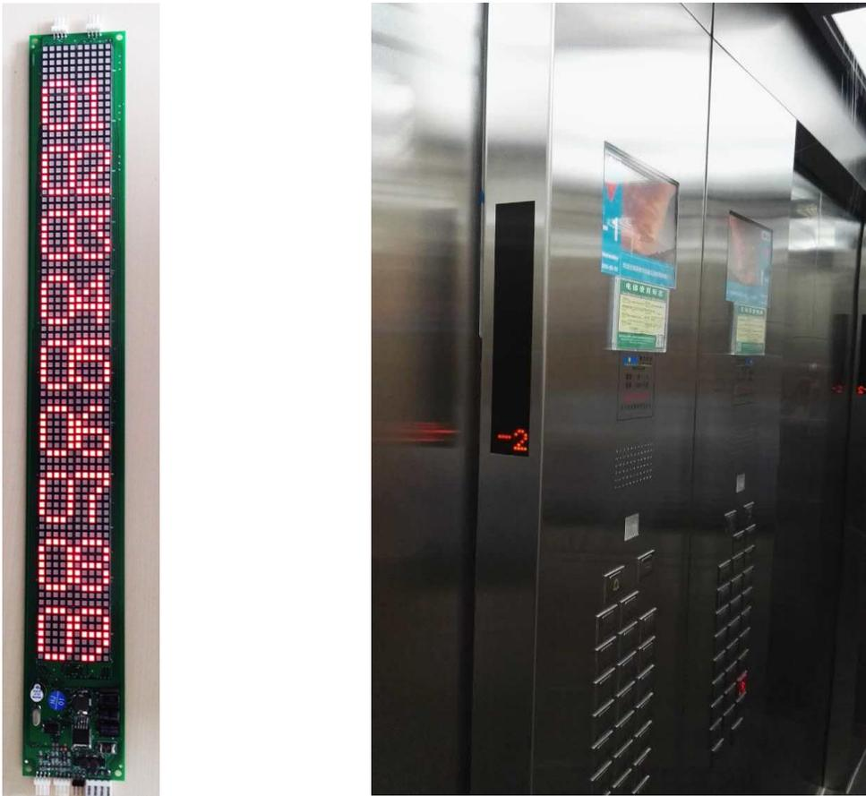
Figure 4.1 Vertical Display Board and Display Board being installed at the Cabin Front Return Panel
