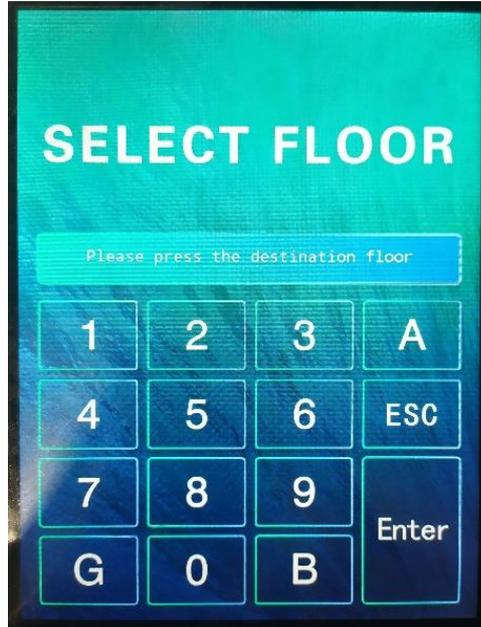
**Figure 3.13 Interface of Floor Selector without Entering Number of Passenger**
