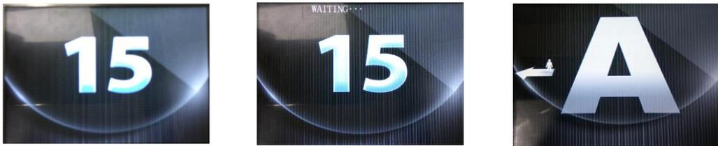
Step.1: Input the target floor Step.2: Waiting for distribution Step.3: Elevator A is assigned, walk to the left.
