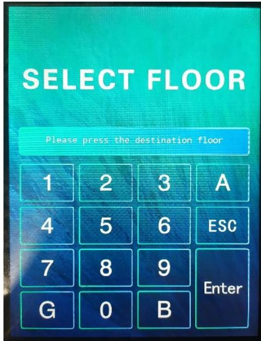
**Figure 3.15 Interface of Floor Selector with Entering Number of Passenger**
