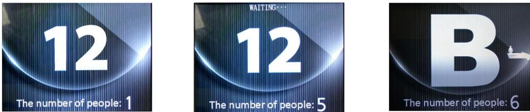
Step.1: Input the target floor    Step.2: Input number of passenger    Step.3: Elevator B is assigned, walk to the right.
