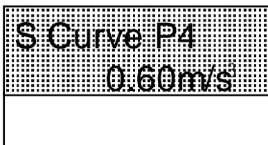
B1,b2,p1,p2,p3 and p4 are used to adjust running curve. Passenger will feel more comfortable by adjusting these six parameters (besides transducer parameters). Parameter is increased, curve slope becomes bigger; parameter is decreased, curve slope becomes smaller. Elevator can meet standards by adjusting them
