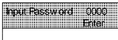
When you enter into input password menu, ' > ' select bit, '^' and ' v ' modify data, if password is right, it will display general parameter menu, otherwise, input password again.
