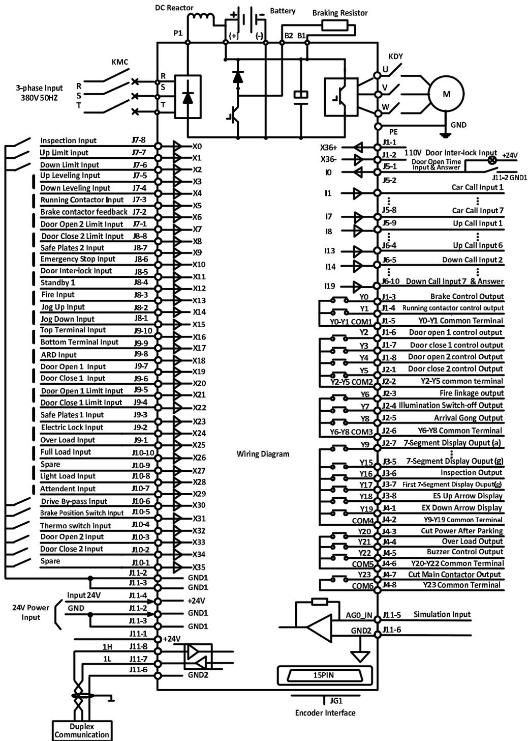
Note: In “Intensive Serial Communication Resolution” of Appendix 6, the terminal with “\*” has no need to wire except X5. For more detail, please check Appendix 6.
