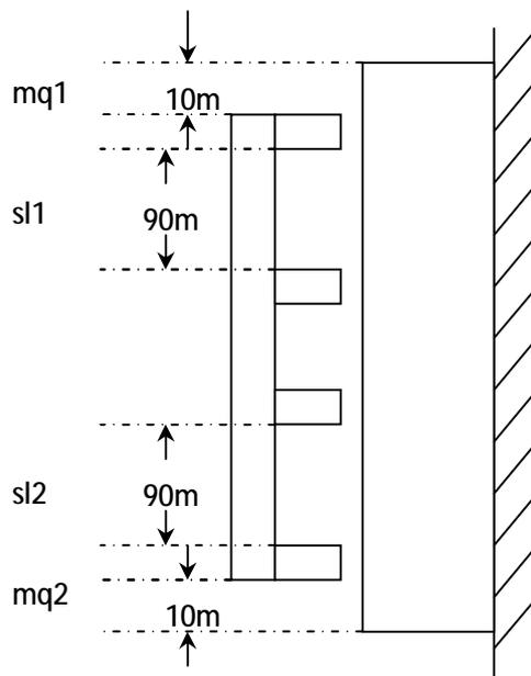
FIGURE F2.3 RE-LEVELING DOOR ZONE SWITCHES POSITION
