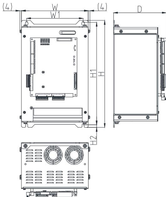
FIGURE 2.3 WITHOUT SHIELD TYPE EXTERIOR DIMENSION
