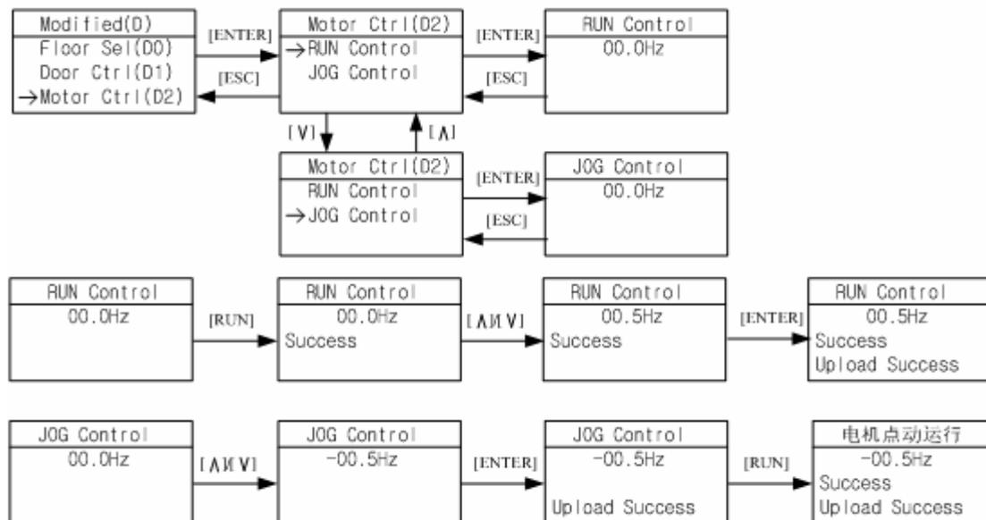
FIGURE 4.8 FLOWCHART FOR OPERATOR TO CONTROL MOTOR RUNNING
