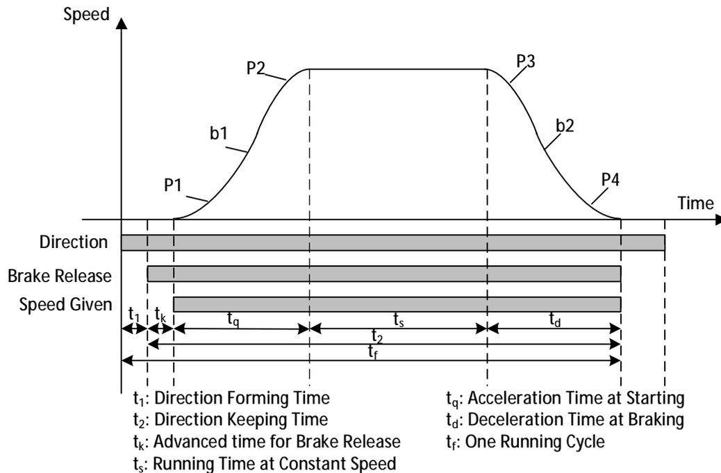
FIGURE 7.6 ELEVATOR RUNNING SPEED CURVE
