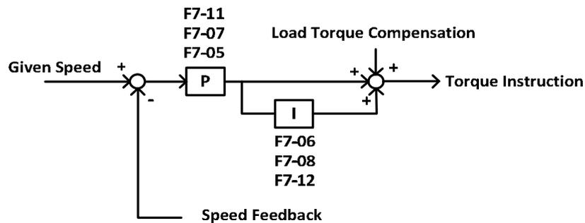
FIGURE 6.12 SPEED ADJUSTMENTS 2
