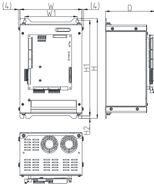
FIGURE 2.3 WITHOUT SHIELD TYPE EXTERIOR DIMENSION
