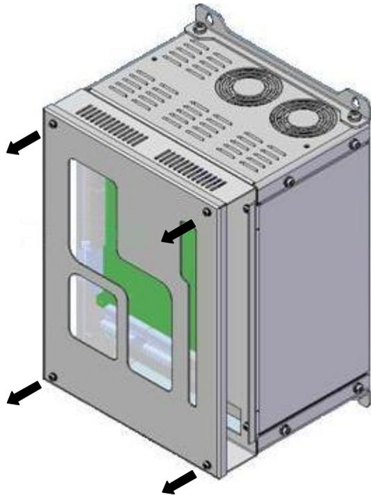
Figure 2.7 Remove terminal cover on shield type
