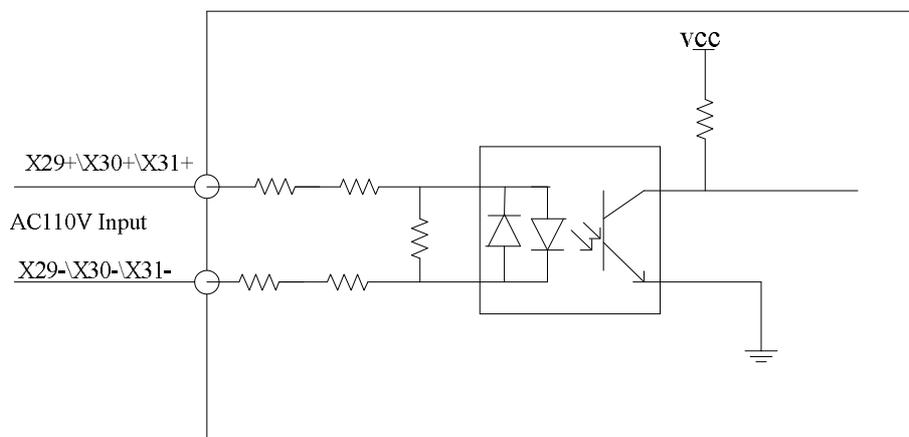
FIGURE 3.9 AC110V INPUT INTERFACE & CONNECTIONS
