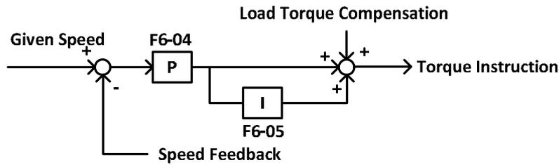
FIGURE 6.11 SPEED ADJUSTMENTS 1
