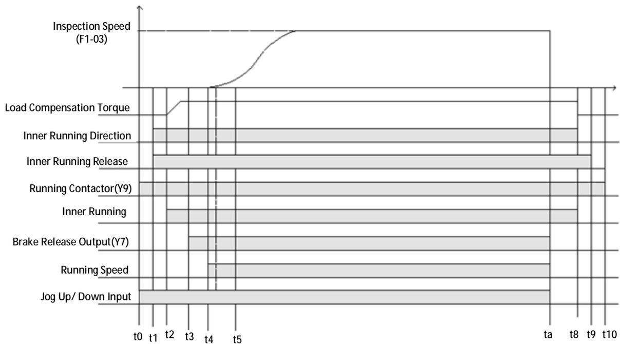
FIGURE 6.4 TIMING DIAGRAM FOR ELEVATOR INSPECTION RUNNING
