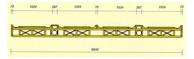
The above dimensions are uninterrupted lane widths only. If there are columns, walls, or passages between lanes, the overall width of lane shall be added as much as the width of them.
